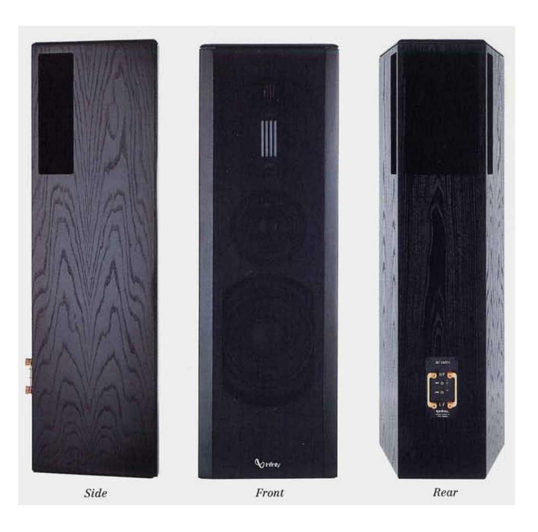
materials and extensive internal bracing makes the Omega trapezoidal enclosure rigid and well-damped, reducing spurious vibration and internal standing waves virtually to the vanishing point. In order to reduce edge reflections which can "smear" the sound, the planar drivers are mounted flush with the front baffle and the speakers' front corners are rounded and tapered.
