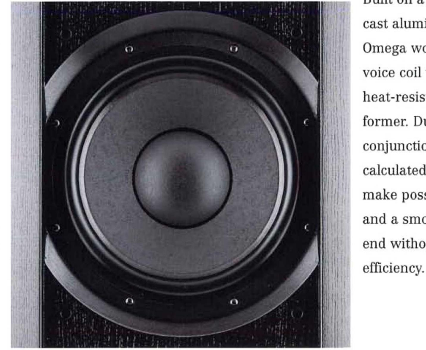
designed and built especially for the Omega is based on William Watkins' revolutionary, yet simple solution to the problem of bass driver design. Built on a non-magnetic, diecast aluminum frame, the Omega woofer employs dual voice coil windings on a heat-resistant fiberglass former. Dual voice coils in conjunction with precisely calculated resonant circuits make possible high output and a smooth, extended low end without sacrificing high
